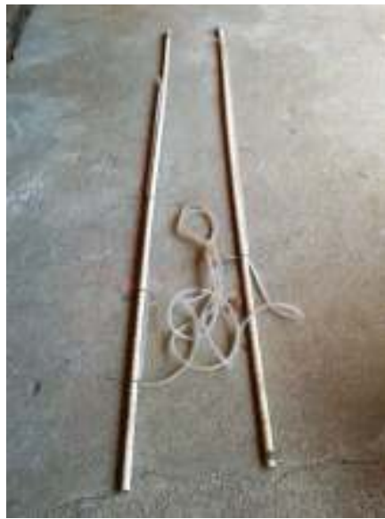
Figure 7: A Completed Water Level
